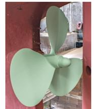
Apply one coat of VELOX PLUS by brush (wet film thickness 100µ, dry film thickness 30µ). Apply it with continuous long brush strokes. Avoid going back and forth on the same spot, as this will soften the METAL PRIMER. As pictured below, full coverage will not be achieved with first coat of VELOX PLUS. The first coat will normally slightly soften the primer, showing some of its green colour.
